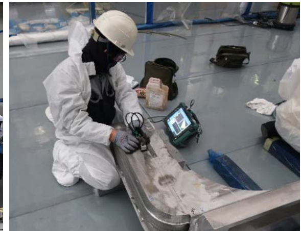
Phased Array UT (NDE) inspection on Shield Plate weldment of NB PSE
