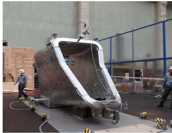
Factory Acceptance Test (Pressure Test) of LPSE 10
