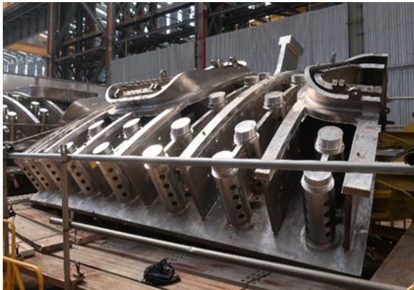
Poloidal Segment #2 (PS2): T-rib, Flexible Support Housing and In-Wall Shielding Support Rib Assembly
