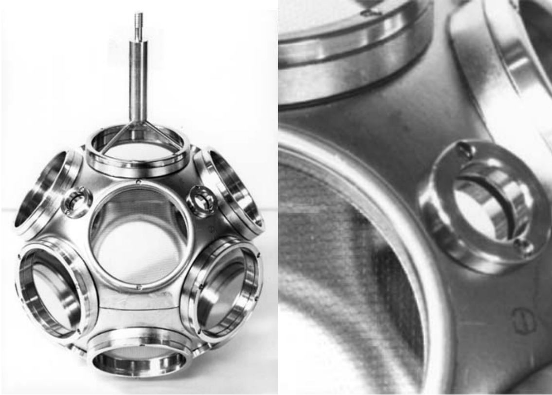
Figure 3.9 Hirsh experiment cathode and close-up of electron streaming suppressor screens.
