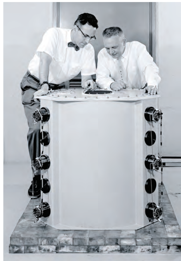
Fred Reines (left) and Clyde Cowan inspect their neutrino detector in 1955, a predecessor to the one they used in 1956 to prove the existence of the elusive neutrino. Forty years later and 21 years after Cowan's death, Reines alone was awarded the 1995 Nobel Prize in Physics for their shared discovery.
