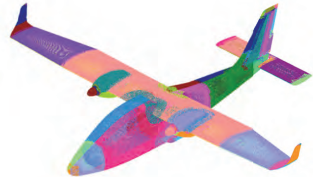
Structured overset mesh
