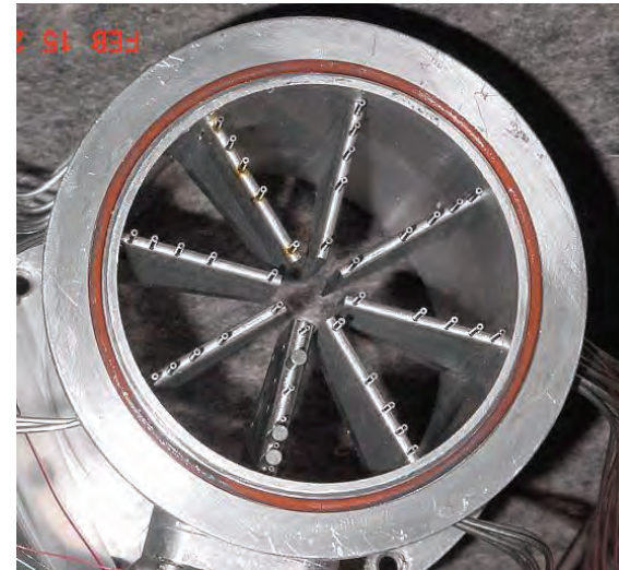
40-Probe Rake Transonic Wind Tunnel Experiment
