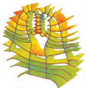
CFD Surface Static Pressure Extracted and Used as Applied Load in FEA
