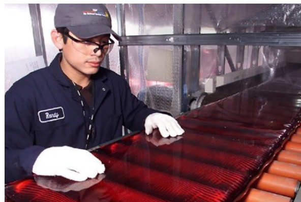
Fig. 20: NIF laser facility (left), continuous strip of laser glass exciting the melter at NIF (right).
