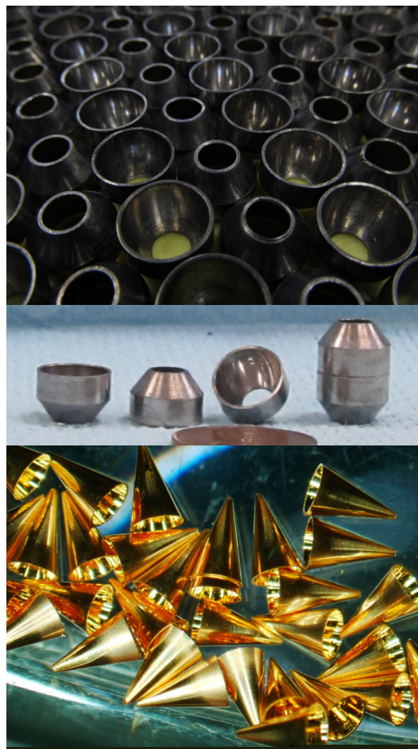
Fig. 10: top - Lead hohlraums produced by swaging at General Atomics. Coin in the middle is a USA penny. Bottom - gold cones produced by electro-forming using a stamped mandrel at General Atomics. Courtesy of General Atomics.
