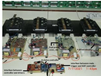
IGBT gate drive controller
