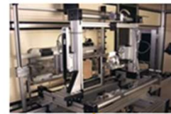
Sample holder for irradiation
