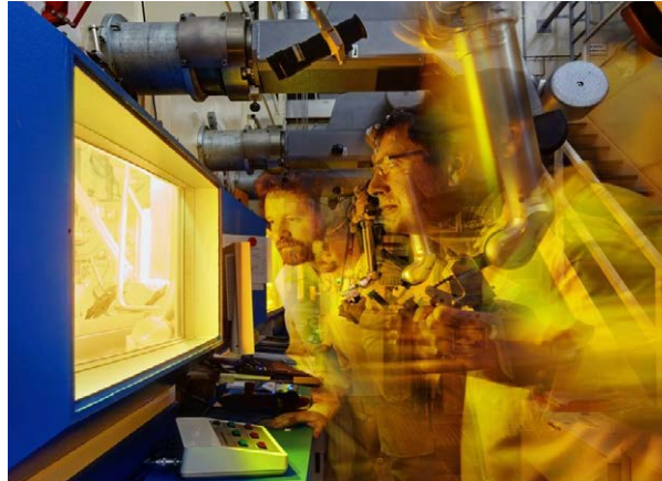
Materials for the vacuum vessel are investigated in the 'hot cells' of the KIT fusion materials laboratory
