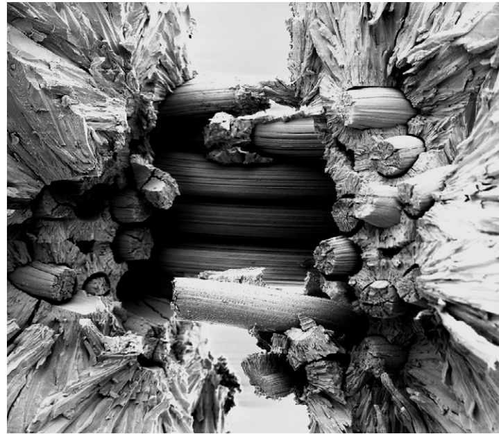
Electron photomicrograph of the fracture point of a tungsten fibre composite. Its use in the fusion reactor could help to better absorb thermal stresses and limit fissuring at the prevailing temperatures.
