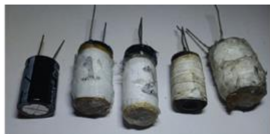
Photo of an electrolytic capacitor with 4 LEC's Made from disassembling an electrolytic capacitor and adding some active material
