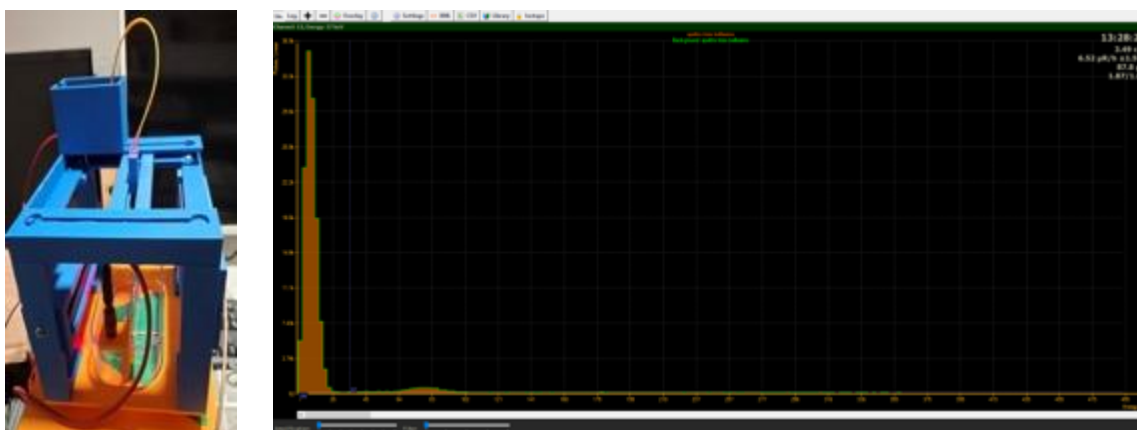
Figure 2. Photo of the reactor (open) in operation and evidence of the bremsstrahlung spectrum of Tritium (the peak at about 11 Kev) acquired by the Radiacode 102 sensor. Acquisition time 13 h 26 m.
