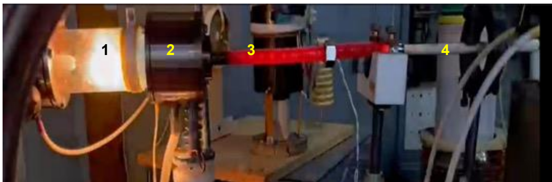
Figure 1. General view of the PVR installation. 1 – reactor anode, 2 – nickel cathode, 3 – stainless steel outlet pipe, 4- measuring thermocouple
