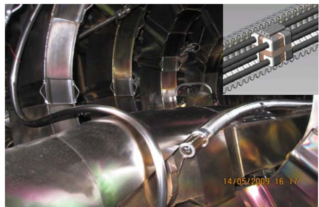
Figure 19: The Toroidal Mirnov array terminating in a special coil set enclosed in a metallised glass tube for high frequency response. The existing poloidal array is in the foreground (bean shaped tube), and CAD detail of a coils set is inset.
