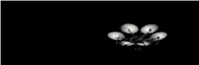
Figure 15: Framed visualization of EBS data showing the scene composition of the second CUAS case, in which the EBS remained stationary and the drone was large with well-resolved rotors. White corresponds to an event; black corresponds to "no data."
