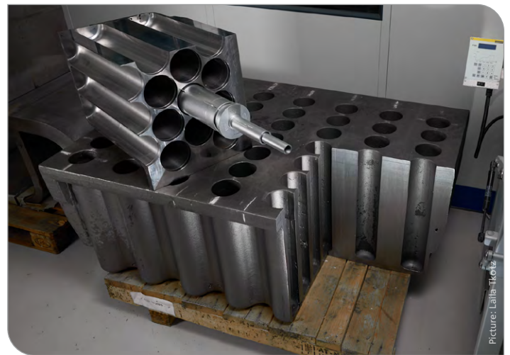
Pin monoblock prototype of the HCPB-TBB
