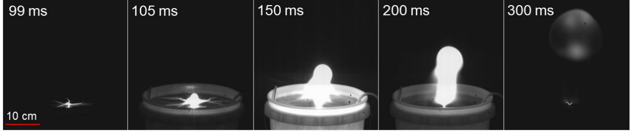
Figure 4.3: A series of images obtained using the Phantom v5.2 high-speed camera from a single plasmoid discharge. A scale bar is included.
