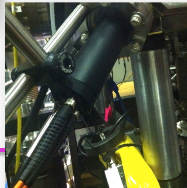
Photodiodes and Spectrometer (Filtered for H_{\alpha} and C_{I-II} , High resolution spectrometer, fiber coupled)
