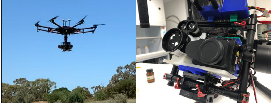
(left) Drone with IR sensing array mounted on gimble; (right) Gimble
