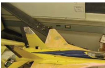
A dynamically scaled flying model of a supersonic business jet configuration
