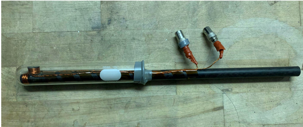
Fig. 3 Photograph of 2-axis B-dot probe used in this study.
