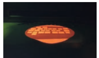
Additively manufactured tungsten parts after the manufacturing process when being removed from the powder bed.
