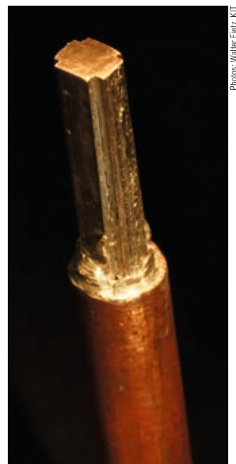
HTS CrossConductor with additional copper cladding
