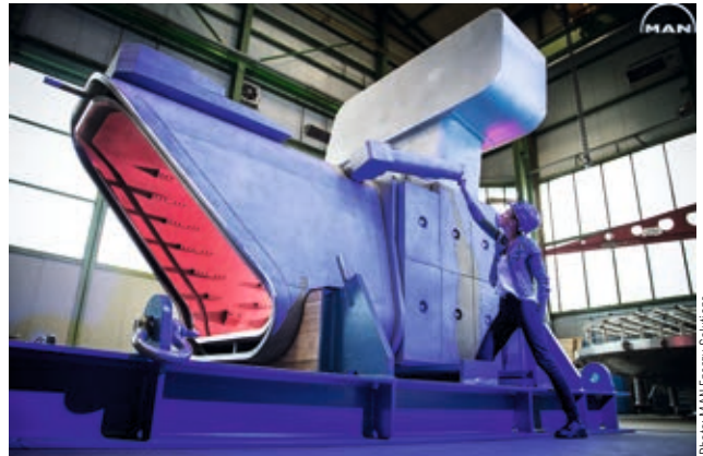
Port for the international experimental reactor ITER
