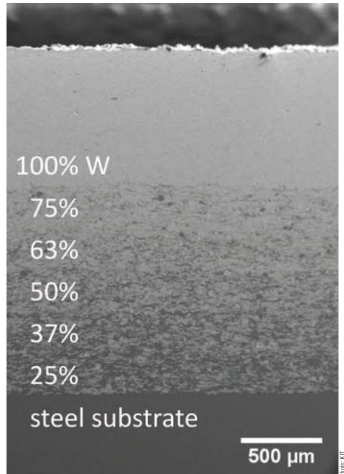
Structure of the protective layer
