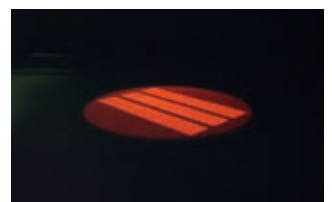
Preheated tungsten build platform during the additive manufacturing process
