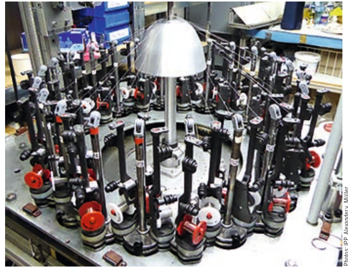
Production of a braid from tungsten wire
