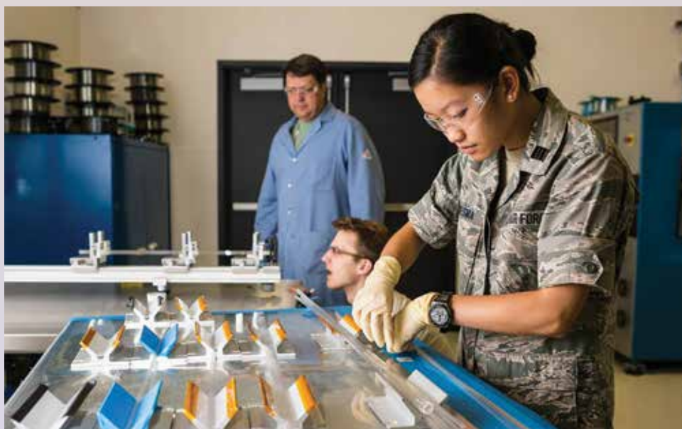
Fabricating photonic crystal optical fibers as part of our research into hollow-core fibers that will dissipate and tolerate laser-generated heat and permit transport of high-power laser light while maintaining good beam quality.
