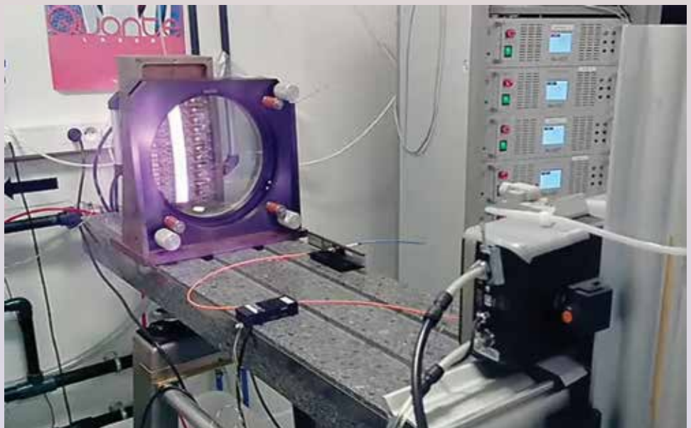
A diode array for our gigashot optical laser demonstrator operating with a power meter at 120-Hz repetition rate.
