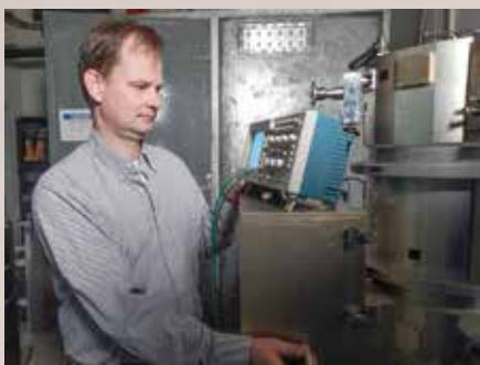
Lawrence Livermore physicist and LDRD researcher Stephan Friedrich adjusts the operating conditions of the superconducting tunnel-junction x-ray detector.
