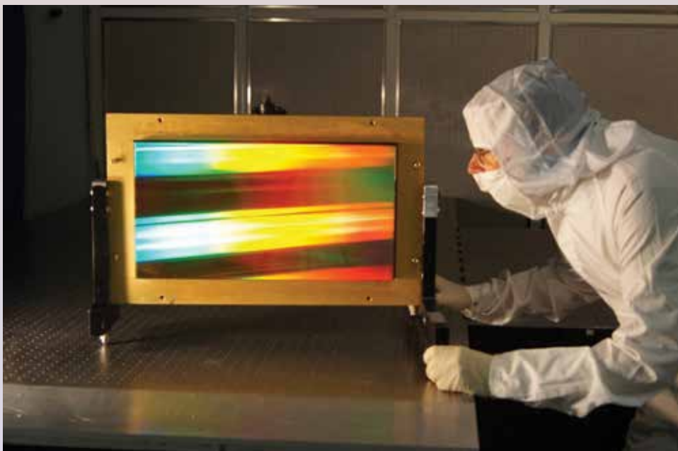
A diffraction grating suitable for a petawatt-class laser pulse compressor. Hafnium oxide is deposited onto an ultralow expansion glass substrate. A 1,480-line/mm groove structure in the hafnium oxide is fabricated using holographic lithography and then coated with a gold layer.
