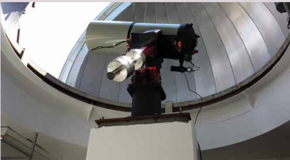
Lawrence Livermore's ground-based observing capability for characterizing orbits of miniaturized satellites.
