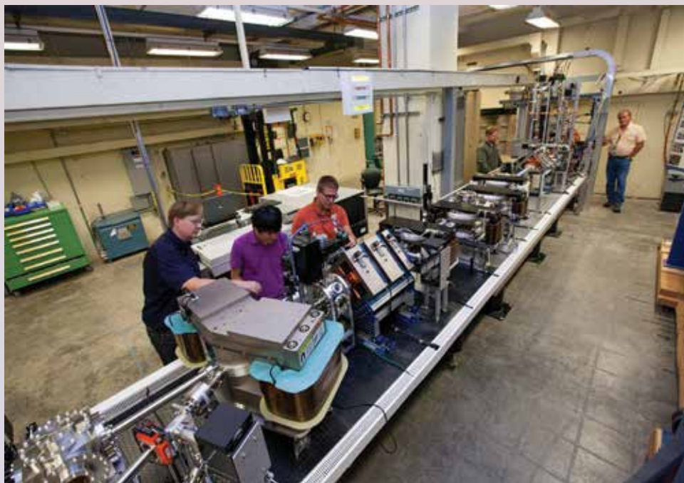
Finalizing installation of our new X-band accelerator at Lawrence Livermore, which can significantly increase the average beam current available from radio-frequency accelerators, and consequently increase the flux available from a variety of beam-based light sources.
