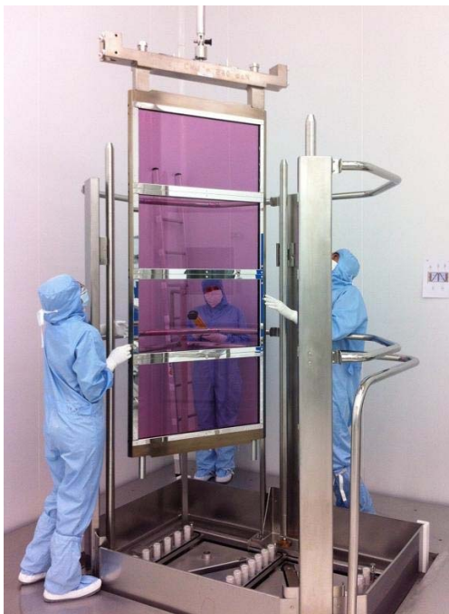
Figure V.4: Mounting of 4 laser slabs, plasma electrode pockels cell and deformable mirror
