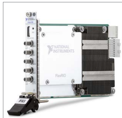
Figure 4 | National Instrument's PXIe-5785 FlexRIO transceiver features user-programmable FPGAs. Photo courtesy of National Instruments.
