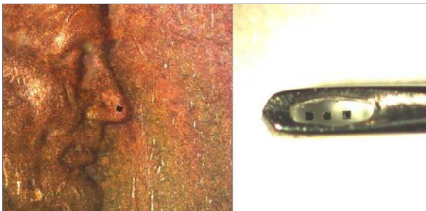
Figure 2 | The 100 micrometer by 100 micrometer dielet reportedly developed by DARPA is intended to act as a hardware root of trust, detecting any attempt to access or reverse engineer the dielet. The SHIELD dielet design consists of passive, unpowered sensors capable of capturing attempts to desolder, delid, or image the circuit; mechanical processes that make the dielet fragile and prevent intact removal from its package; a full encryption engine; and advanced near-field technology to power and communicate with the dielet. Photo courtesy DARPA.
