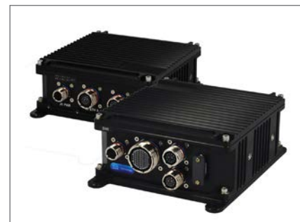
Figure 1 | Curtiss-Wright's DuraNET 30-2020 and DuraMAR 5915 are examples of rugged embedded switch and router systems.
