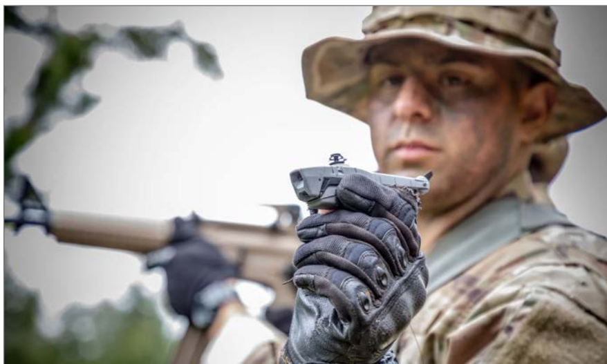
Figure 1 | The Black Hornet PRS from FLIR Systems provides the nonspecialist dismounted soldier with immediate covert situational awareness, according to FLIR Systems.
