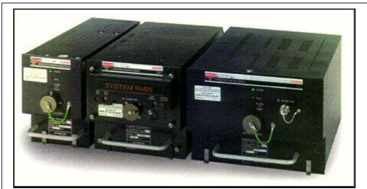
Figure 1.9L - RFU (left), SDU (centre) and HPA (right)
