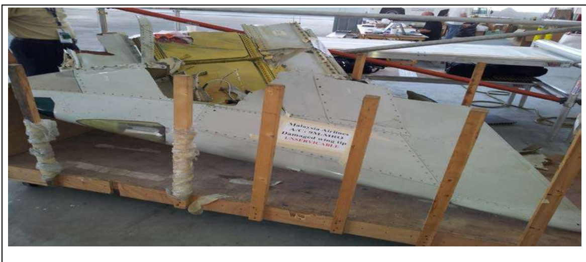
Figure 1.6B - Damaged Wing Tip
