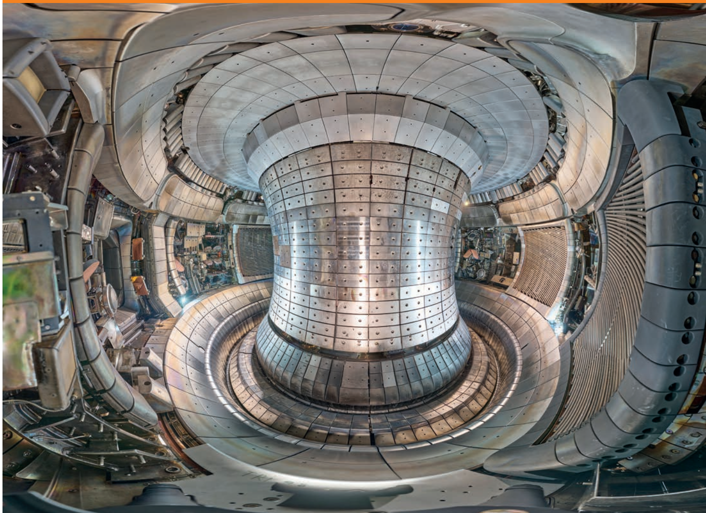
Fish-eye view into the interior of the ASDEX Upgrade vacuum vessel in August 2024, following the installation of the new upper divertor (photo: V. Rohde).
