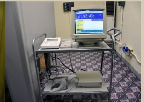
Hot Cell 2 Dispensing of I-131 in container with computer control measurement
