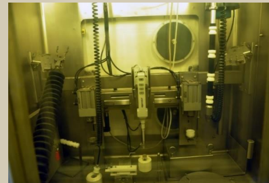
Hot Cell 2 Dispensing of I-131 in container with computer control measurement
