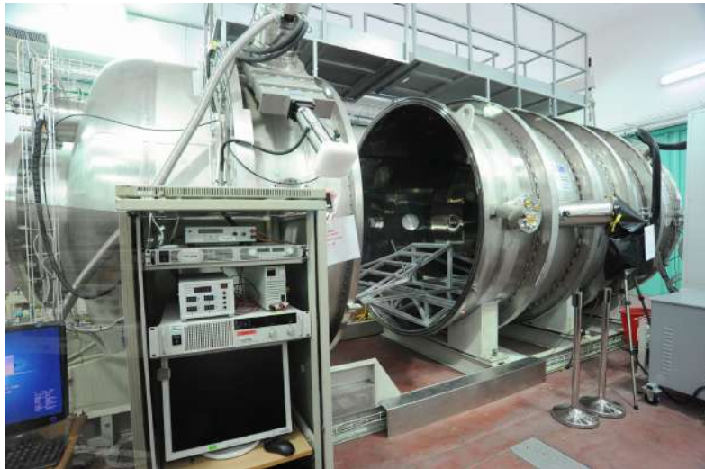
Electrical Test Firing Chamber
