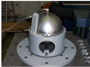
Propellant Tank mounted on shaker for Vibration Testing
