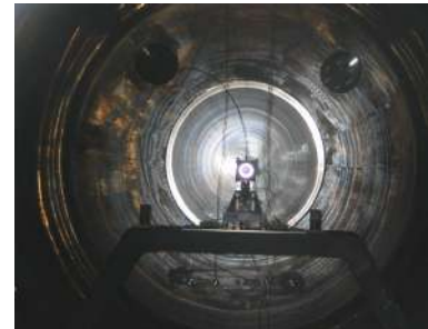
IHET 300 Thruster installed inside Test Firing Chamber
