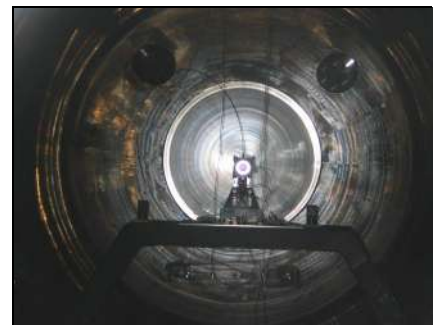
Thruster installed in Firing chamber
