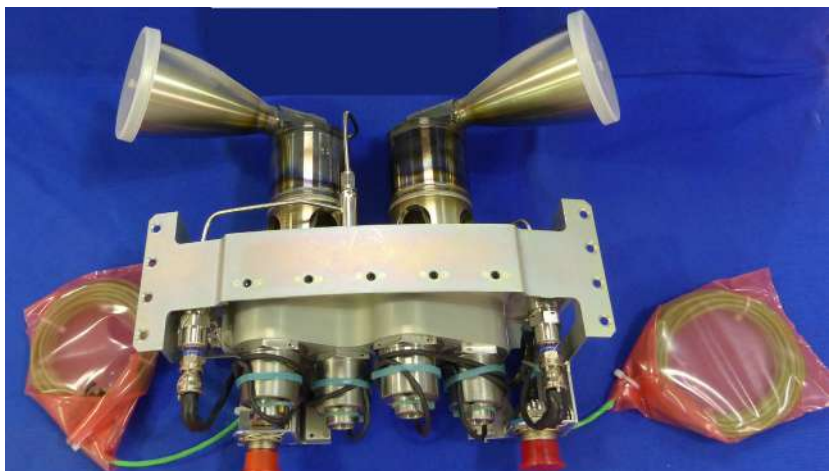
200N Thrusters integrated in the RACS cluster containing valves, pressure transducer and electronic driver
