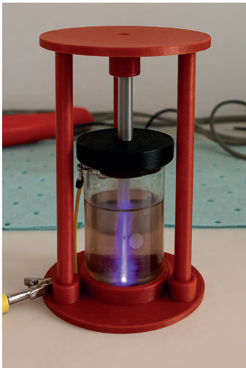
3 The VDBD bubbling device for liquid waste sterilization.
