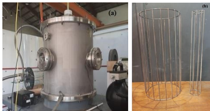
Fig.1. (a) upgraded IR-IECF device and (b) the electrodes in cylindrical geometry
