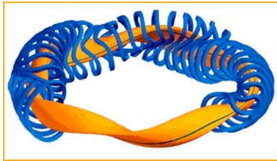
Fig. 4-3. W7-AS modular non-planar coils and plasma.
