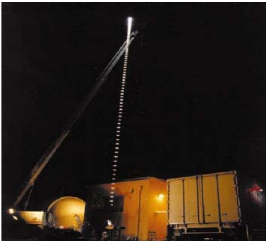
Figure 14. Time-Lapse Photo Of A Lightcraft Undergoing An Outdoor Vertical Flight Test (From AFRL Press Release)
