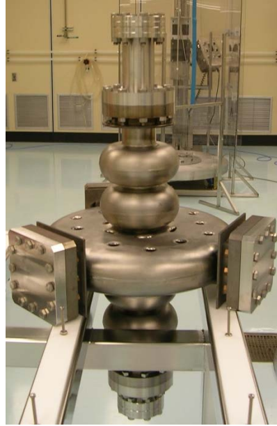
Figure 17: The 2.1 GHz 5-cell SRF accelerating module with a PBG cell.
