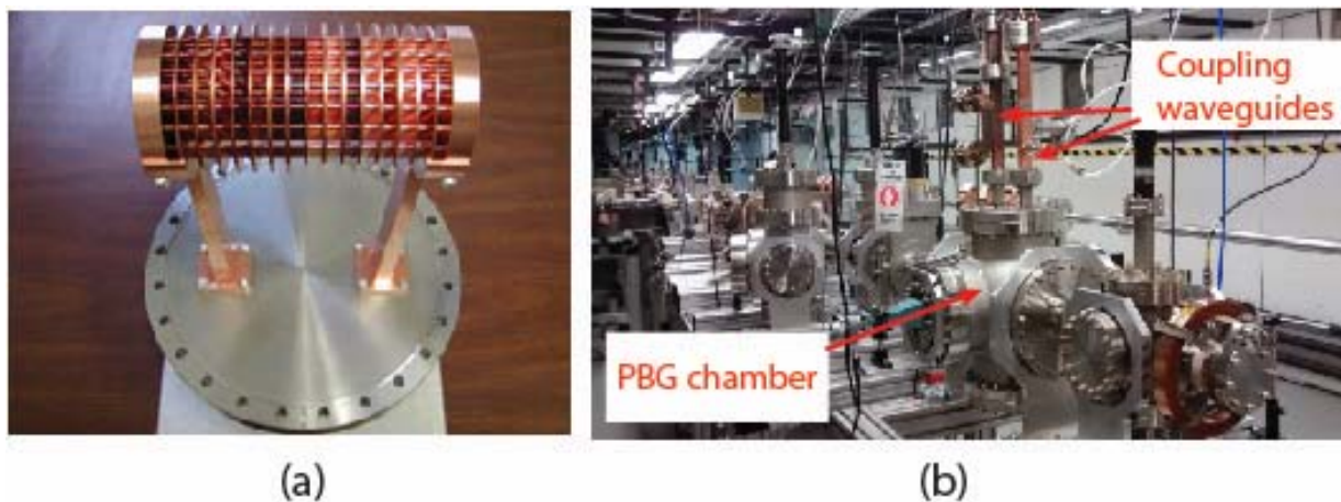
Figure 12: The 16-cell PBG structure installed on a 10-inch stainless steel flange (a); the 10-inch experimental chamber with the PBG structure installed on the beamline at AWA (b).
