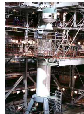
Orbus 21D being stacked on launch pad
