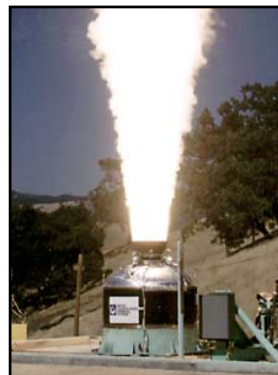
Orbus 21D Static Test
