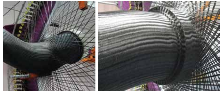
Figure 4 Asymmetrical braiding of a curved-shape demonstrator
