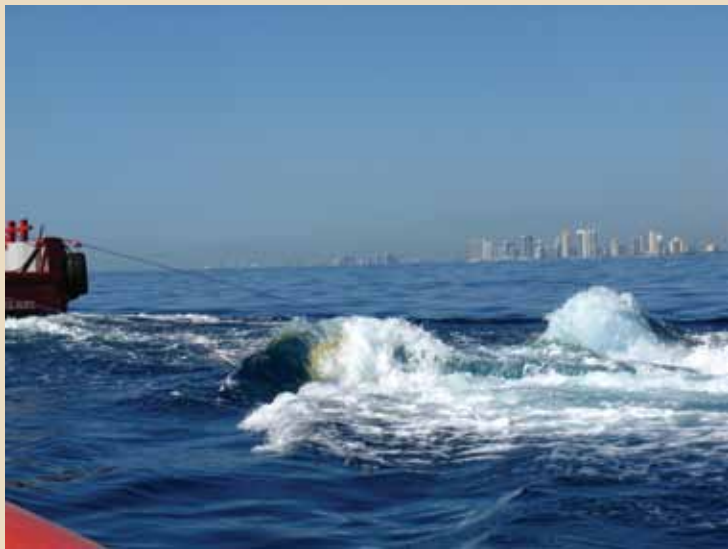
Figure 4 Photo of a wake created by chute with short trailing distance
