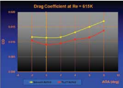
Figure 3 Comparison of drag measurement results of smooth and TLJT airfoils
