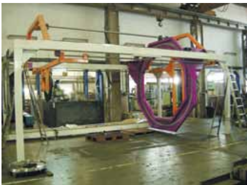
Figure 3 Partial assembly of a multi-axis braiding machine
