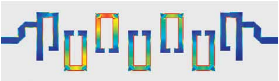
Figure 9 Simulated RF current densities flowing in the metal-strips of the filter
