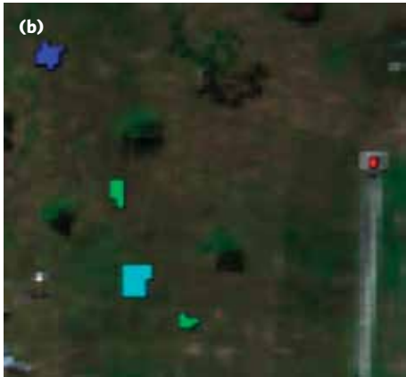
(a) Input image of a scene and (b) output image obtained after material detection was carried out. An experiment was carried out where some known targets (Materials A, B and C) were planted in the scene as shown in (a). The material detection algorithm managed to flag out the materials present (Material A: Blue; Material B: Green; Material C: Cyan)
