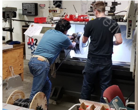
Figure 42 The 30-turn coil is wound manually at HyperJet with the help of a large lathe.
