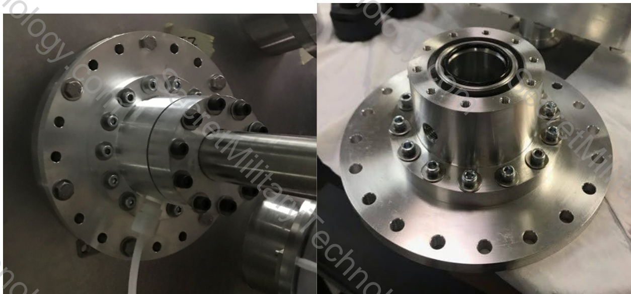
Figure 58 Diagnostic rod seal assembly
