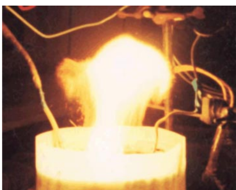
Figure 11. Development of the interaction between the luminous object envelope and the wire segment with an insulation defect.
