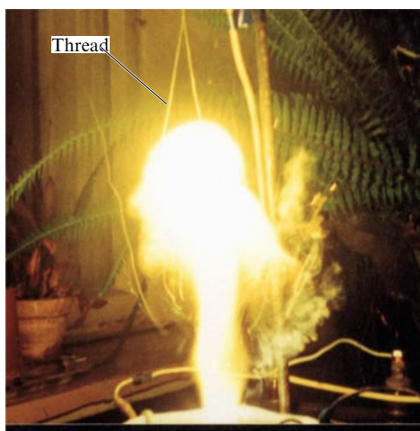
Figure 16. Nichrome wire ring suspended by thin threads is in the nascent luminous object. The metal ring melts at one site. The threads do not change their properties.
